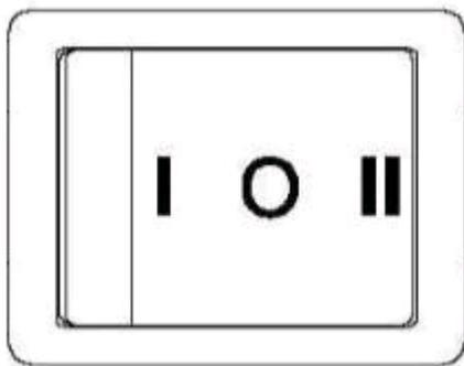
Press the side of the rocker switch to choose the appropriate speed **Low (I)** or **High (II)**
